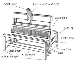
FIGURE 1: ASSEMBLED 4-SHAFT LOOM
